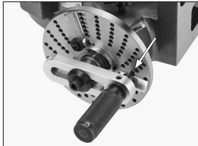
Figure 18. Setting the pin in the last hole.
