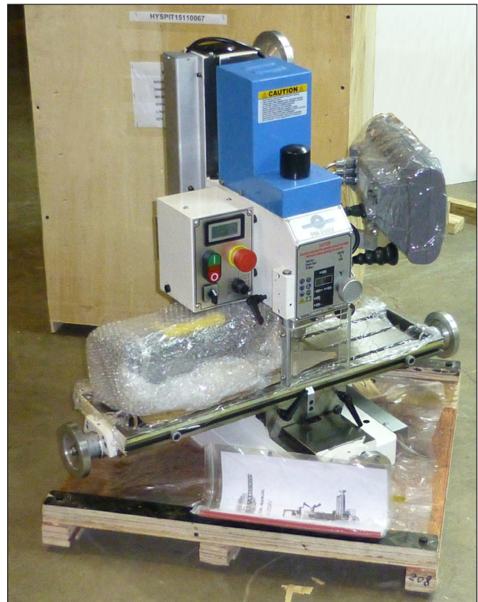
Figure 1-1 Mill ready for lifting
